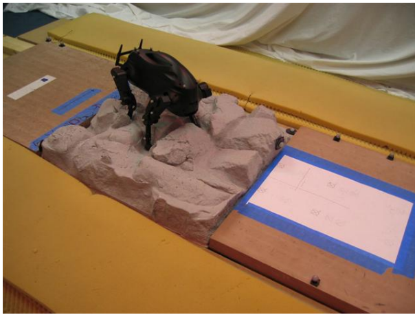
Fig. 5. LittleDog robot crawling over rough terrain.
