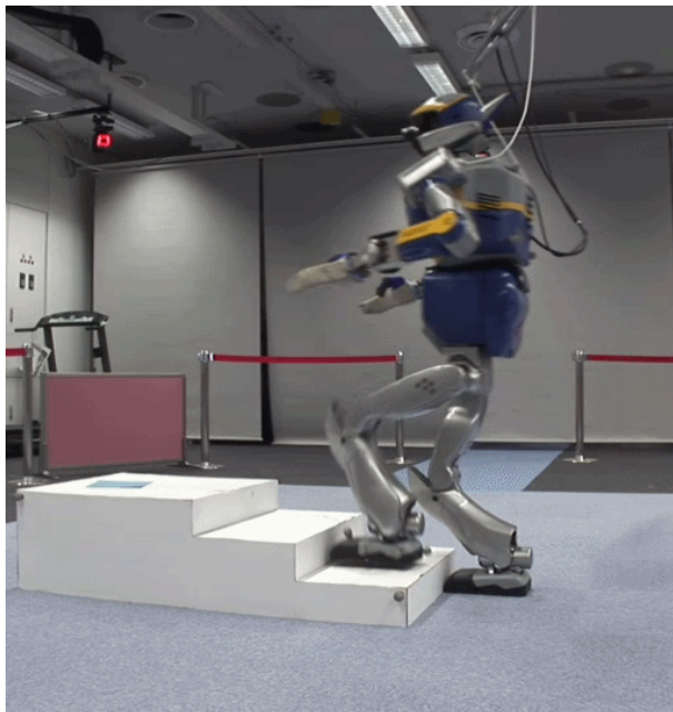
Fig. 1. HRP-2 humanoid autonomously walking up a set of stairs.
